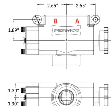
**Manual** shifted model with knob pulled out activates "A" Port. Knob pushed in activates "B" Port.
